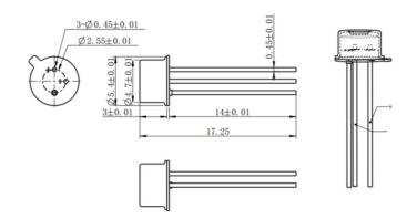
VD-0940P-025W -1N-3A0 (Channel array 1x4, substrate AIN, Package 1x4)
