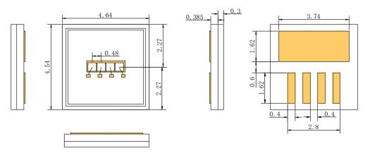
VD-0940P-025W -10-3A0 (Channel array 1x8, substrate AIN, Package 1x8)
