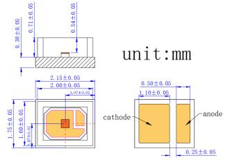
VD-0940P-025W -3A-3A0 (Channel array 1X1, Substrate CuAg, Package 2016)
